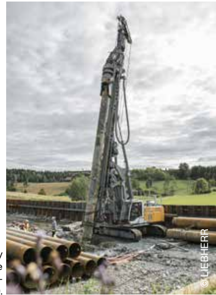
The Liebherr LB20 rotary drilling rig is equipped with the Teufelberger-Redaelli non-rotation-resistant rope Evolution P9 .
